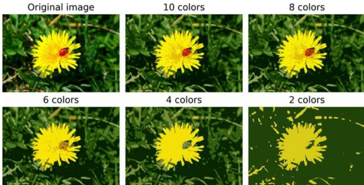
Figure 9-12. Image segmentation using k -means with various numbers of color clusters
