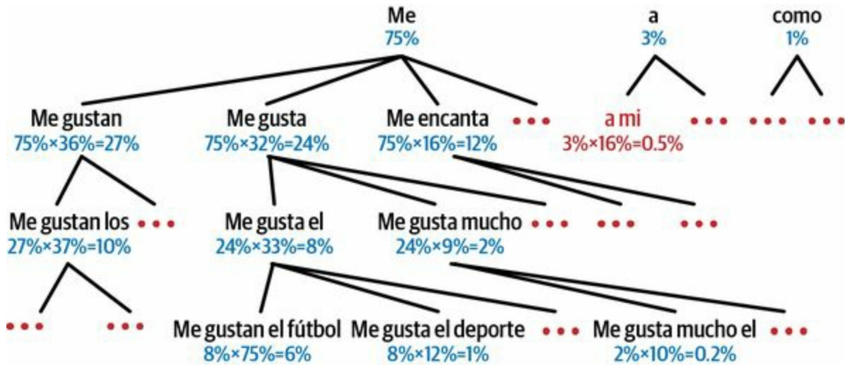
Figure 16-6. Beam search, with a beam width of 3
