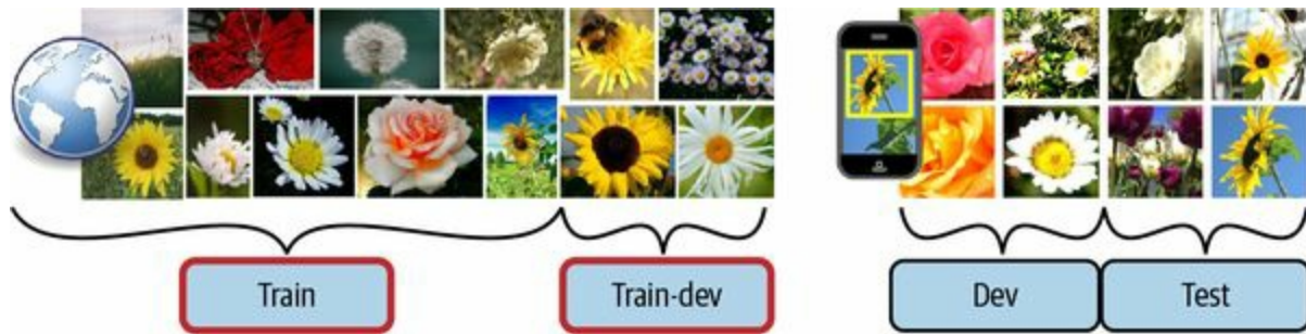
Figure 1-26. When real data is scarce (right), you may use similar abundant data (left) for training and hold out some of it in a train-dev set to evaluate overfitting; the real data is then used to evaluate data mismatch (dev set) and to evaluate the final model's performance (test set)
